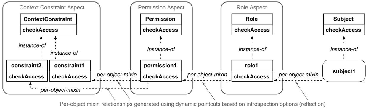
**Figure 3: Example of an executable model generated from the RBAC DSL**
