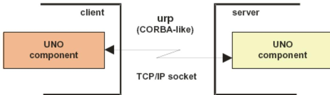
Figure 2: Client-/Server-Communications with UNO Components Using TCP/IP Sockets and the CORBA-like Protocol “urp” (UNO Remote Protocol). [Flat05-1, p.7]
