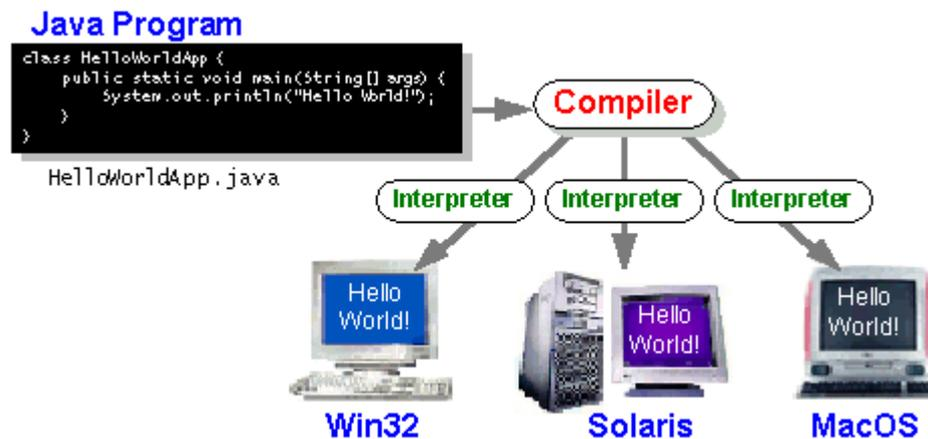
Figure 2: Java byte code can be executed on any platform [Java01]
