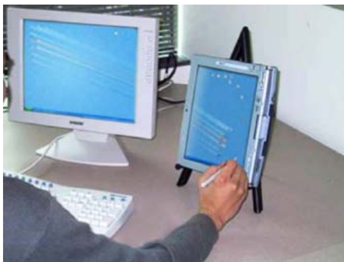
FIGURE 35: DRAG AND DROP ACROSS MULTIPLE DEVICES [BAUDISCH, ET AL., 2003]. THROWING DOCS IS LEANED ON THIS TECHNOLOGY
