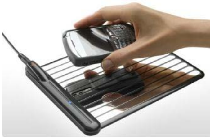
FIGURE 34: WILDCHARGE INDUCTIVELY RECHARGES A MOBILE DEVICE [WILDCHARGE, 2008]
