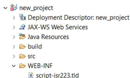
Figure 5: Example of a new created dynamic web project
