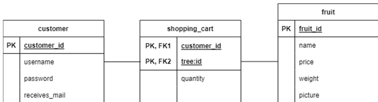
Figure 16: Entity Relationship Model of the database tables
