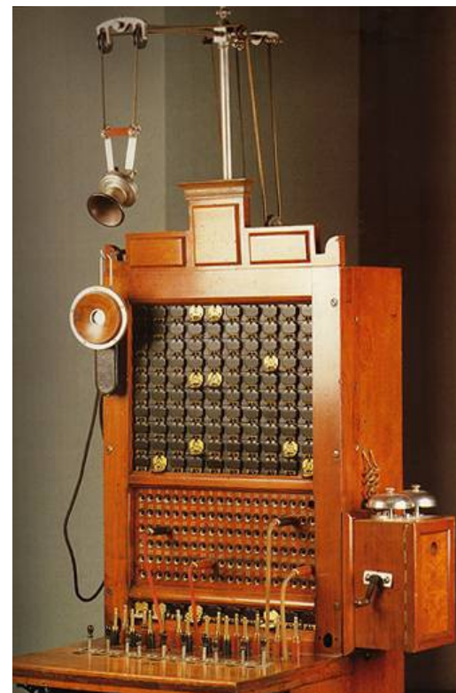
"Switchboard" with 100 ports
